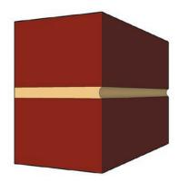
Wherever possible it is beneficial to tool the mortar to a "bucket handle" finish as this provides the best durability and weathertightness.
